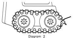
Chain or tie ends of track together with installation tool. Continue backing machine until ends of track are between wheels (Diagram 3). Remove chain or rope.
